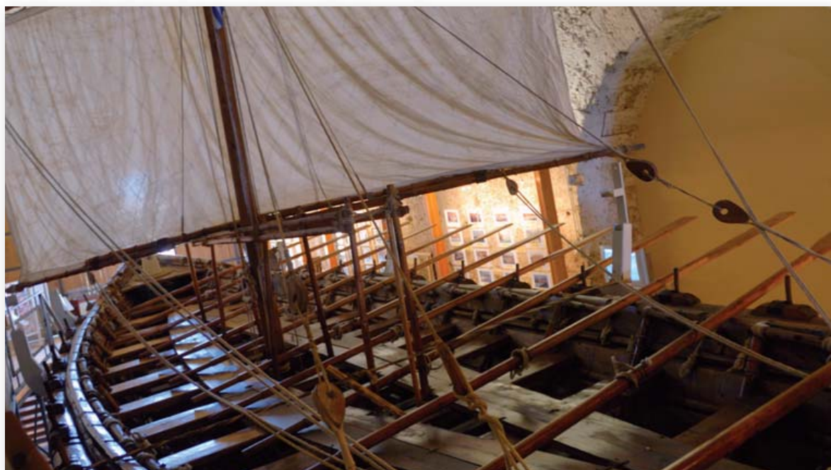
A reconstructed Minoan vessel, now in the Maritime Museum in Chania, Crete, showing the sail footed with a boom, a distinctive feature of many Minoan ships. The gangway is mounted upon the rowing benches, providing height during boarding actions. Note that in the absence of dedicated storage, the oars are laid across the gunwale. (Alamy)
