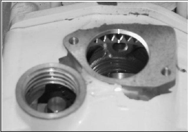
Figure 10-87 Camshaft Gear and Gear Cover Marks
