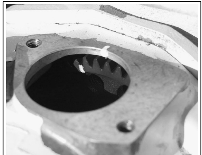
Figure 10-89 Camshaft and Gear Cover Mark
