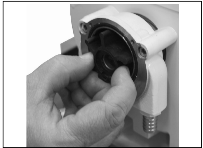
Figure 10-7 Seawater Pump Impeller
