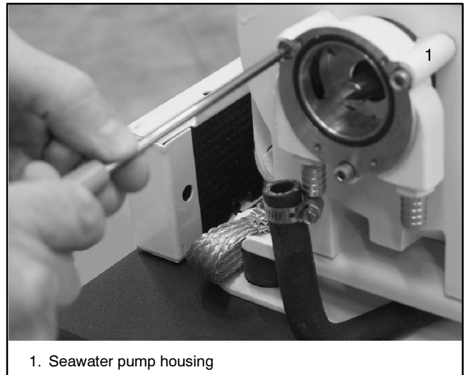
Figure 10-8 Seawater Pump Housing
