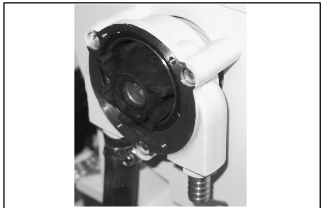
Figure 10-23 Seawater Pump Impeller
