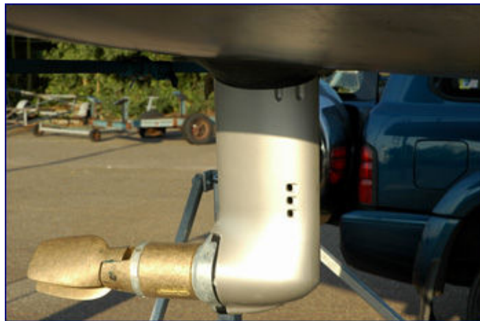
Figure 1 – Sail Drive Configuration
