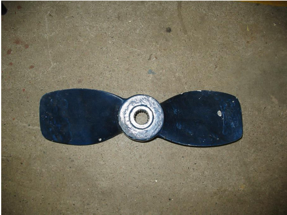
Figure 3 - Two Bladed Fixed Propeller
