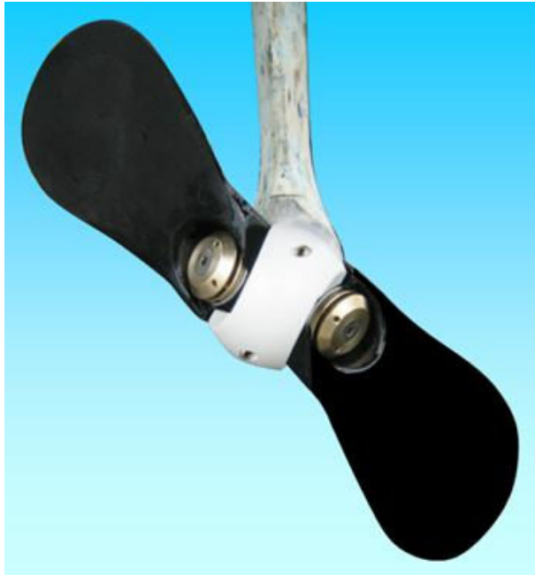
Figure 26 - SDC Prop with blades open
