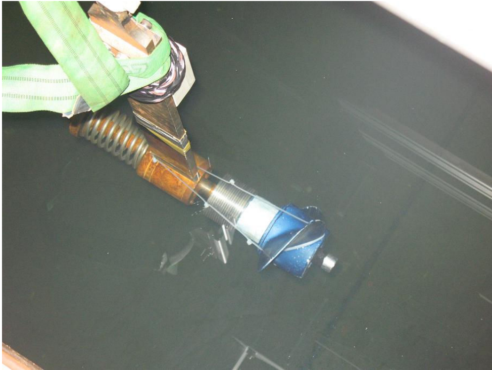
Figure 22 - Cable Tied Propeller
