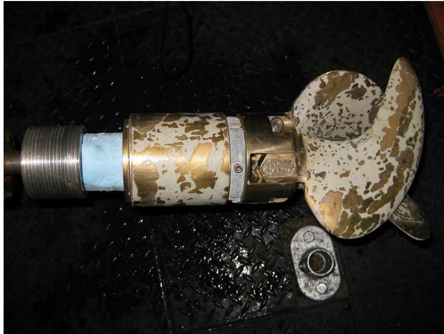
Figure 19 - Three Bladed Prop with washer
