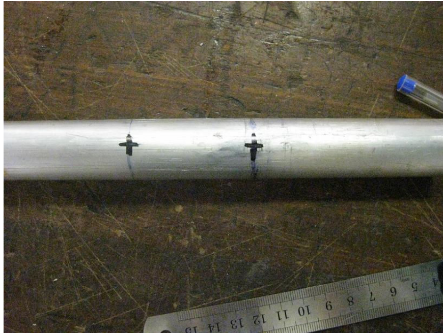
Figure 17 – Marked drilling positions
