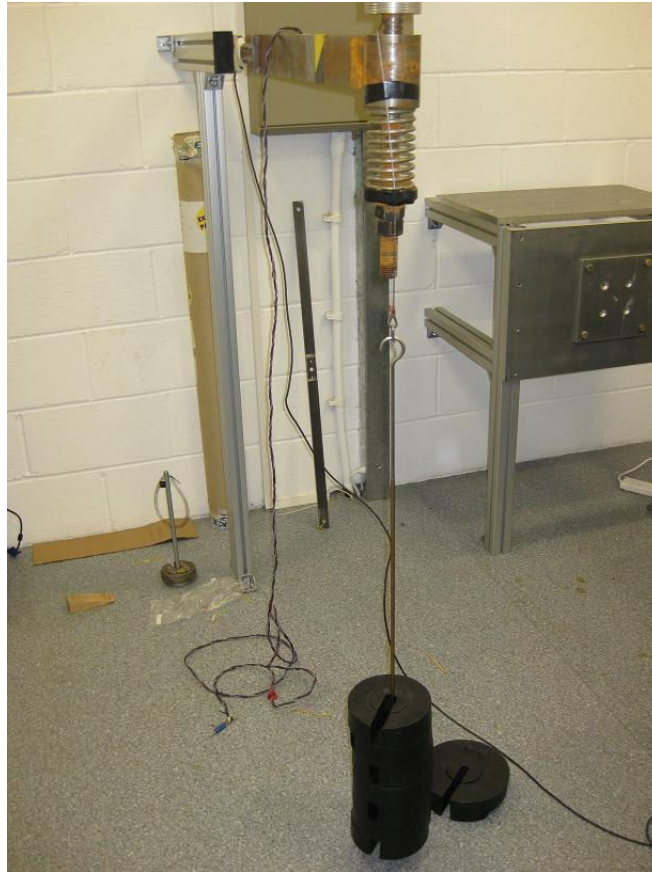
Figure 21 - Test Rig undergoing calibration
