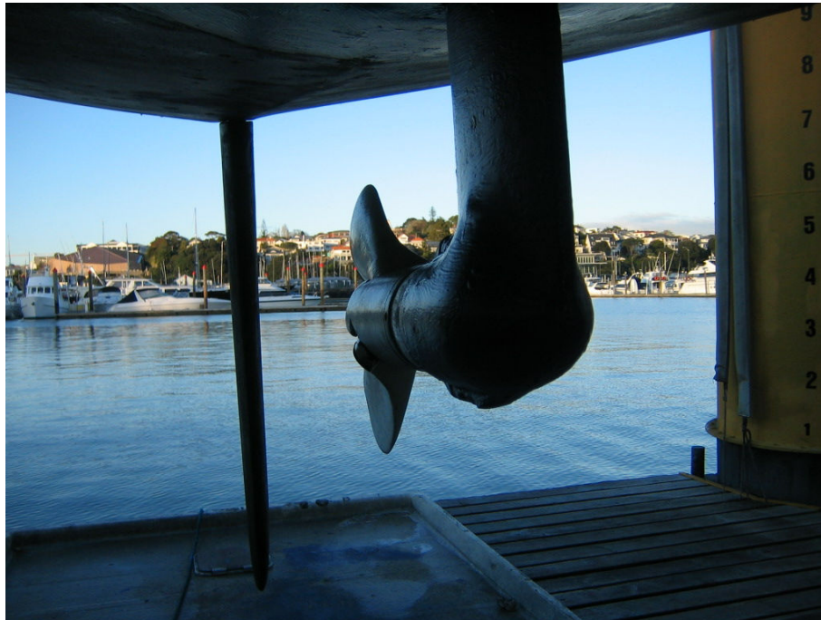
Figure 25 - SDC Prop Folded & Feathered away in sail position
