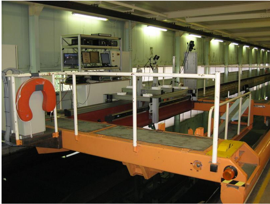
Figure 8 - Tow Tank Test Carriage
