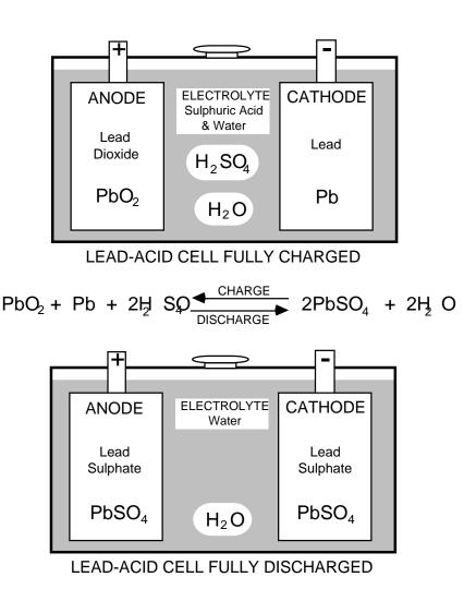
Figure 1- An electrochemical schematic of the lead-acid cell.
