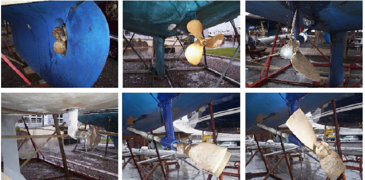
Fig. 1. A variety of propulsion configurations commonly found on sailing boats. Clockwise from top left: fixed three-blade in aperture behind long keel; fixed three-blade on exposed shaft well behind fin keel; feathering three-blade on shaft, fin keel; folding two-blade, deployed; folding two-blade, folded; folding three-blade, folded, on sail-drive strut behind high aspect-ratio keel.
